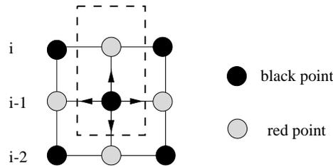
FIG. 2.1. Data dependencies in a red-black Gauss-Seidel algorithm.
