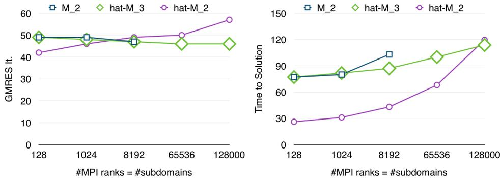
FIG. 4.8. **Linear 3D Cube**  $\Omega = [0, 2] \times [0, 1] \times [0, 1]$ ; see Table 4.2 for a problem description.
