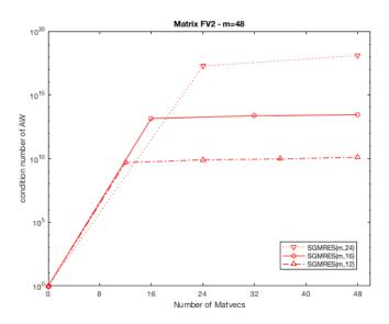
FIG. 5.3. Impact of block size s in SGMRES(m,s). Condition number of  $AW_{sj}$  with the matrix fv2 using m = 48 and s = 12, 16, 24.
