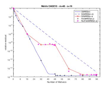
FIG. 5.10. Comparison of fixed and variable s-step GMRES. Convergence curves with the matrix cage10 using m = 48 and s = 16.
