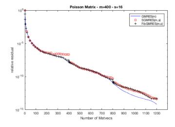
FIG. 5.9. Comparison of fixed and variable s-step GMRES. Convergence curves with the large Poisson matrix using m = 400 and s = 16.
