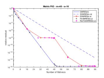
FIG. 5.5. Comparison of fixed and variable s-step GMRES. Convergence curves with the matrix fv2 using m = 48 and s = 16.
