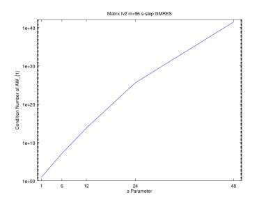
FIG. 5.4. Condition number of  $AW_s$  as a function of s. Results with the matrix fv2 using m = 96.
