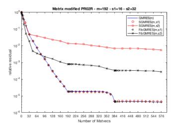
FIG. 5.14. Comparison of fixed and variable s-step GMRES. Convergence curves with the modified PR02R matrix using m = 192 and s = 16, 32.
