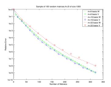
FIG. 5.1. Comparison of Traditional and Non-Traditional variants of m-step GMRES(m). Mean error curves with a sample of 100 random matrices using m = 8, 16, 32.
