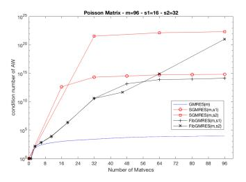
FIG. 5.8. Comparison of fixed and variable s-step GMRES. Condition numbers of  $AW_{l_j}$  with the Poisson matrix using m = 96 and s = 16, 32.
