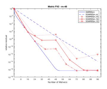
FIG. 5.2. Impact of block size s in SGMRES(m,s). Convergence curves with the matrix fv2 using m = 48 and s = 12, 16, 24, 48.
