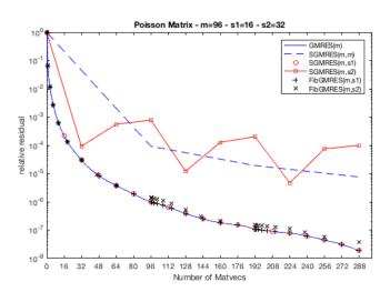
FIG. 5.7. Comparison of fixed and variable s-step GMRES. Convergence curves with the Poisson matrix using m = 96 and s = 16, 32.
